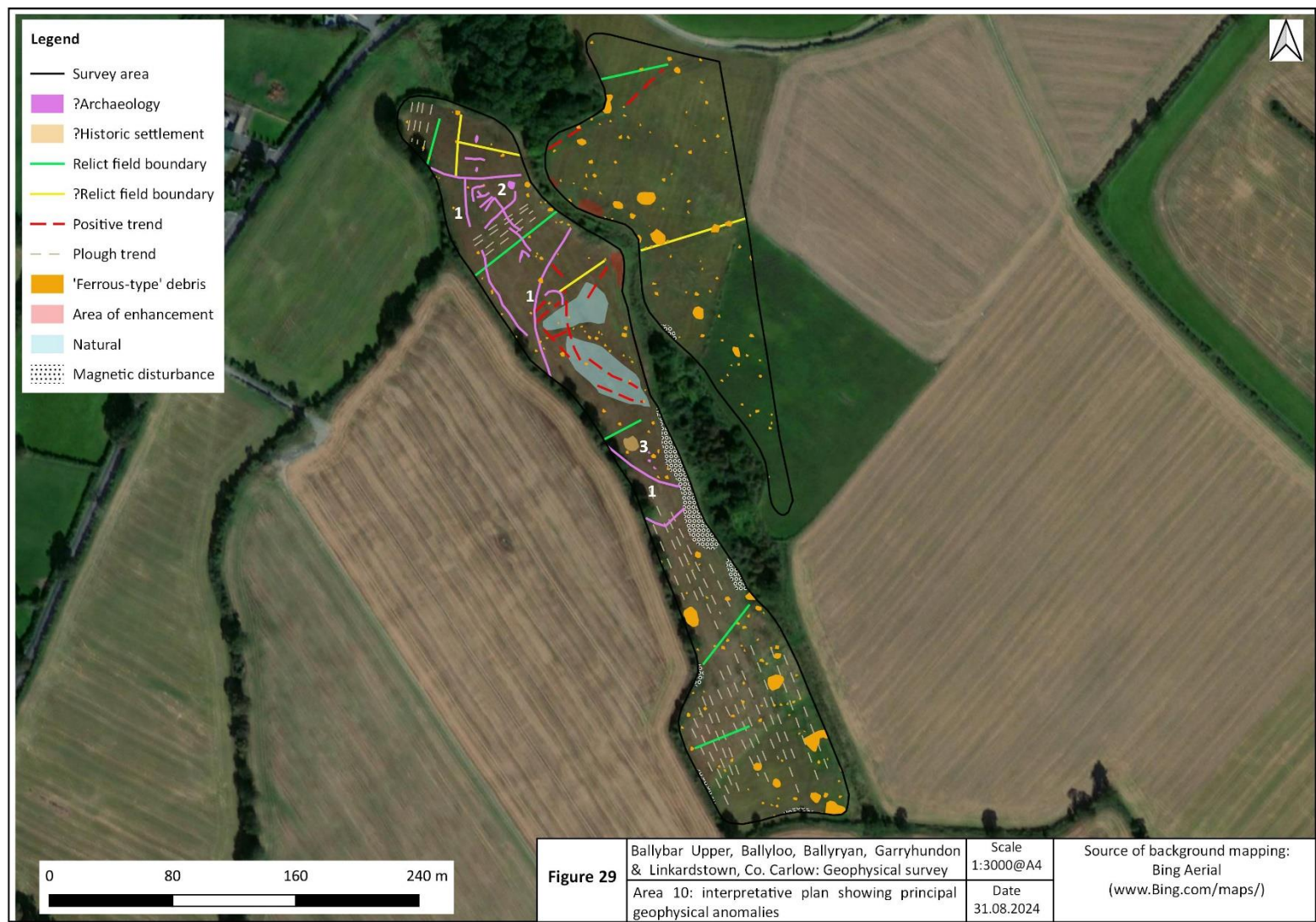
Figure 29. Area 10: interpretative plan showing principal geophysical anomalies.
