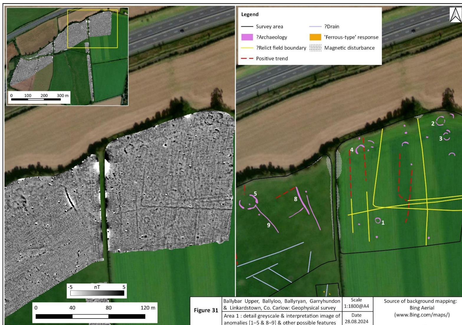
Figure 31. Area 1: detail greyscale and interpretation plan of anomalies [1–5 & 8–9] and other possible features.
