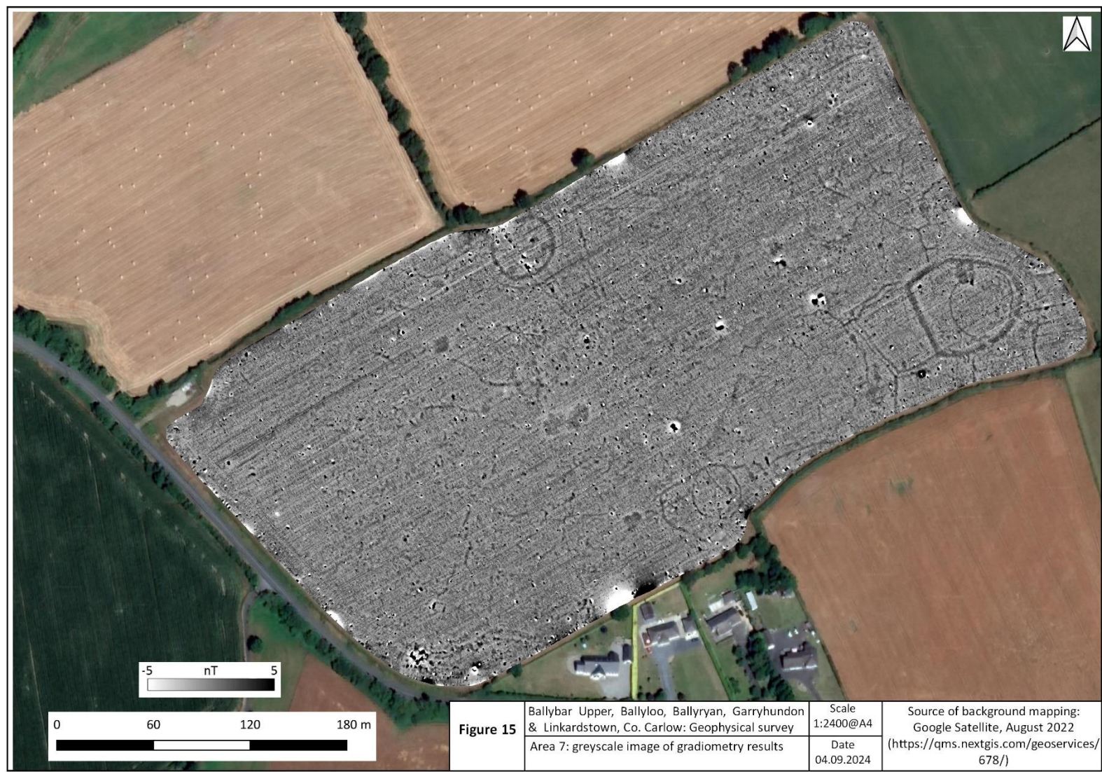
Figure 15. Area 7: greyscale image of gradiometry results.
